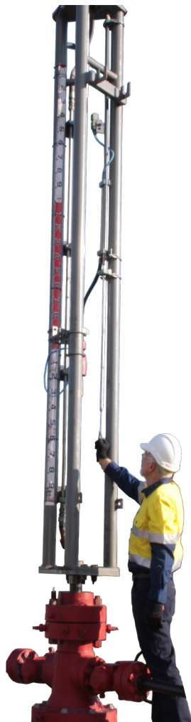
Adjusting top sensor from ground level
